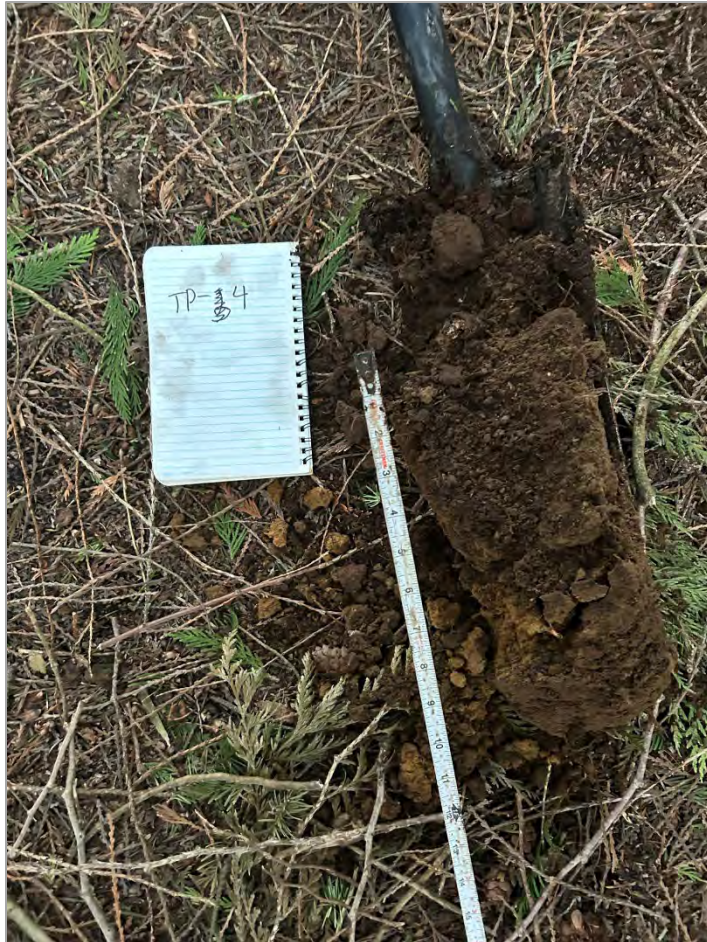
Photo 3. Soil profile of TP-4
