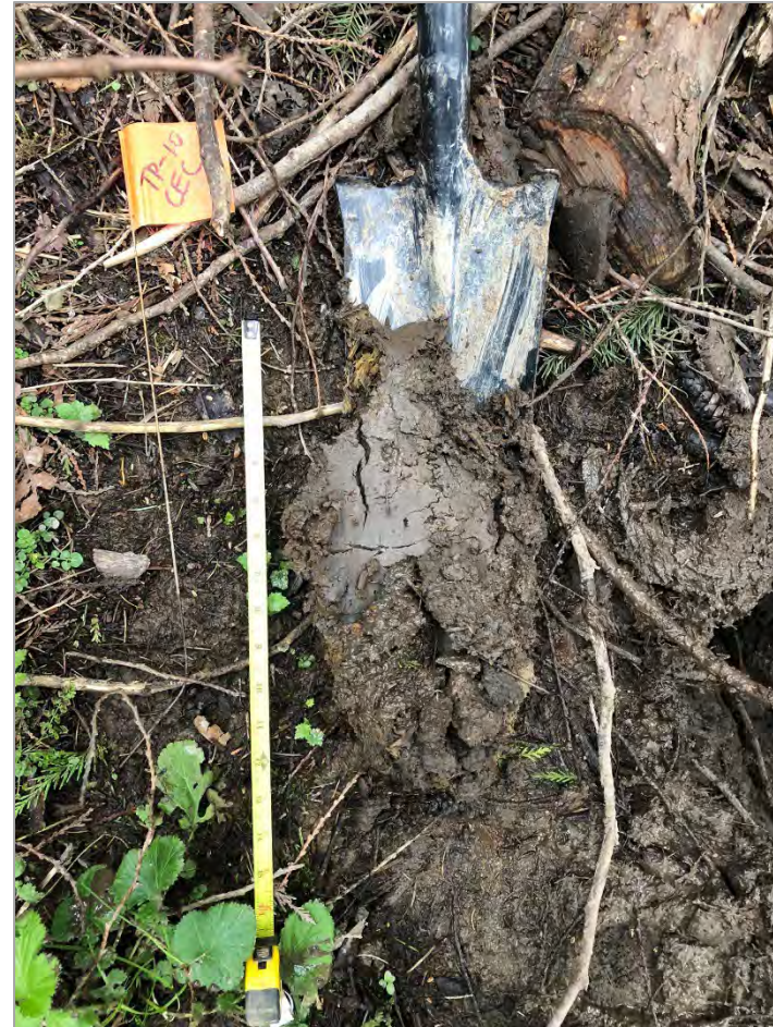
Photo 6. Soil profile of TP-10
