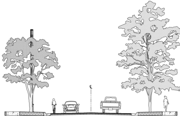
Small Cell Facilities within the Amenity Zone
